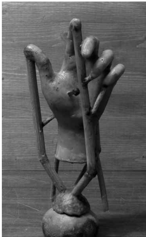
Figure 37.15. After the insertion of the chaplets (by A. Pacini, 2011).
